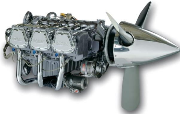
Figure 1.0 Typical General Aviation Six Cylinder Engine Spark Ignition
