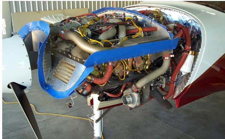
Figure 2.0 Installed 350 BHP Turbocharged Engine
